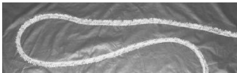
Figure 14 Abrasion uniforme de la surface
